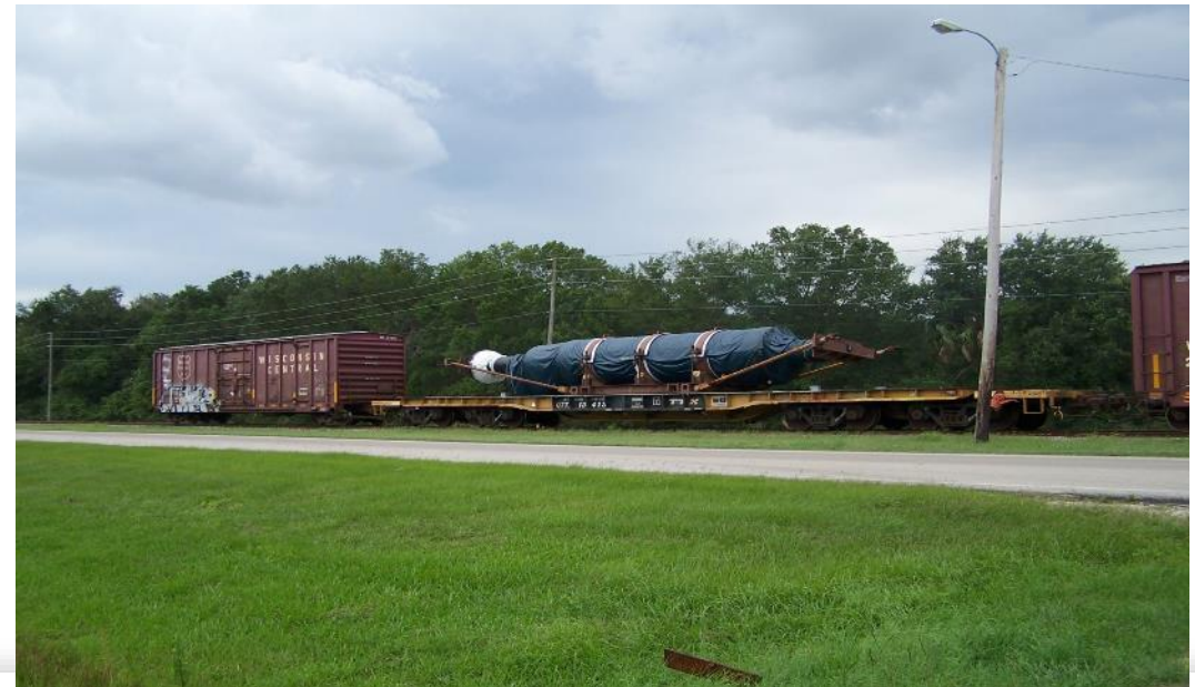
Generator Rotor 395,000 lb. 50' long x 8' diameter (October 2009)
