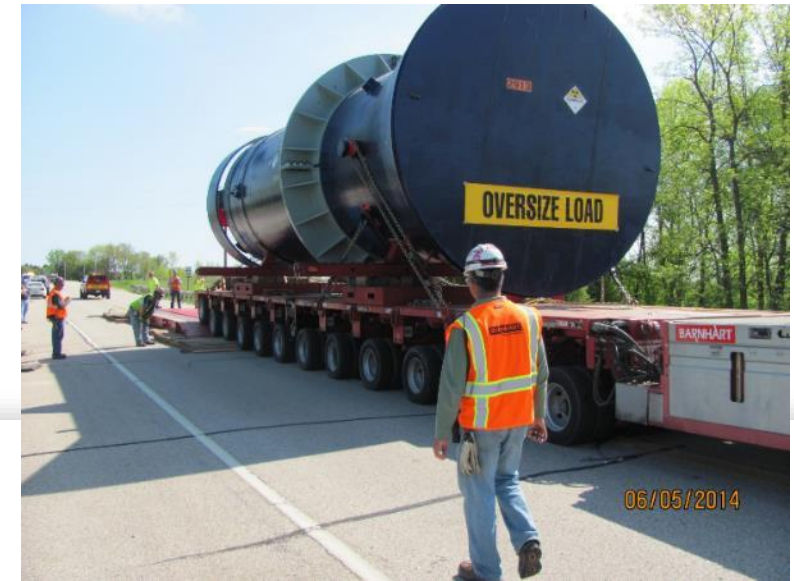
Steam Generator Shipping Near Kewaunee
