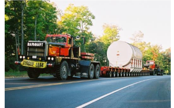
Big Rock Point Reactor Pressure Vessel Heavy Haul Photo courtesy of Barnhart Crane & Rigging
