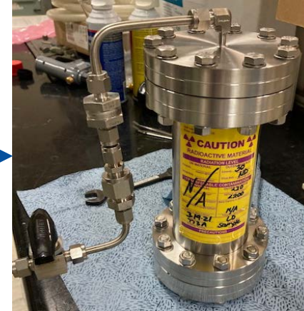
MURR sample sealed in mini-canister for radiolysis testing
