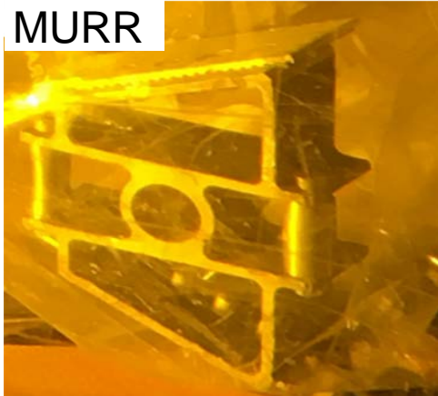
MURR Missouri University Research Reactor (MURR) element – wet storage
